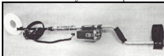
Control housing mounted under pole
